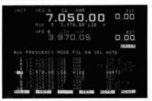
Unique Spectrum Scope. Continuously indicates all signal activities and DX pileups with your operating frequency in the center. Selectable horizontal frequency spans of ±50, ±100, and ±200KHz for each side of the frequency you're listening to. Vertical range indicates relative signal strengths. A contester's dream!
